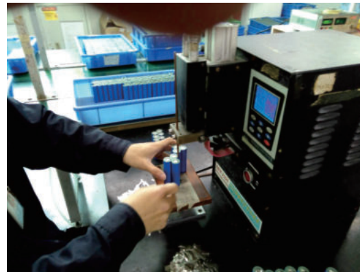
Battery welding machine
