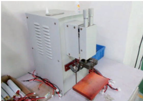
Battery welding machine
