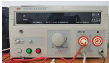
High Voltage Test Equipment
